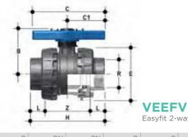
Easyfit 2-way ball valve with BSP threaded female ends
