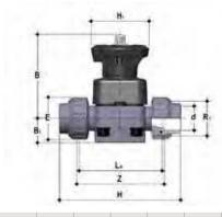
**DKUAV** DIALOCK<sup>®</sup> diaphragm valve with female union ends for solvent welding, ASTM series
