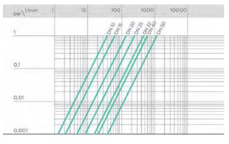
E - L-port ball valve: 0°/270° - Diverting
