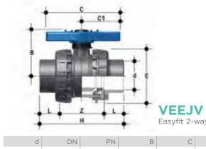
Easyfit 2-way ball valve with female ends, JIS series
