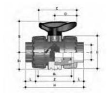
VKDLV DUAL BLOCK<sup>®</sup> 2-way ball valve with female ends for solvent welding, BS series
