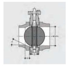
Before proceeding with the installation of the stubs, check that the bore of the fittings has sufficient clearance to allow the valve disk to open correctly. Also check the maximum coupling distance for the liner. Before proceeding with the installation of the FK valve, check that the bore of the stub allows the correct opening of the disk.
