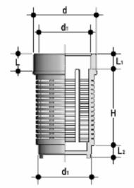
Suction strainer with male and female ends for solvent welding to foot valve VZ
