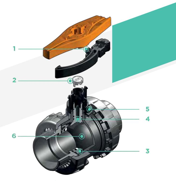
Innovative Easyfit quick release handle made up of a central hub firmly coupled with the stem valve and dual spoke grip that can be released from the hub with a simple operation and used as a ball seat adjustment tool and as a union nut tightening tool thanks to the hooked insert that, perfectly adapting to their external profile, allows the handle to transform into a wrench to control union nut rotation
