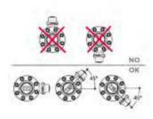
Make sure that the valves installed on the system are suitably supported for their weight.
