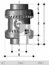
Easyfit ball check valve with female ends for solvent welding, metric series
