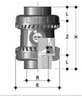
**SXENV** Easyfit ball check valve with female ends, NPT thread
