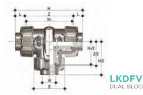
DUAL BLOCK® 3-way ball valve with BS parallel socket threaded ends, L bore.
