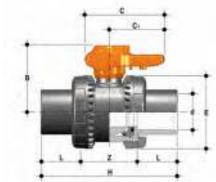
Easyfit 2-way ball valve with female ends, JIS series
