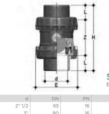
**SXEJV** Easyfit ball check valve with female ends, NPT thread
