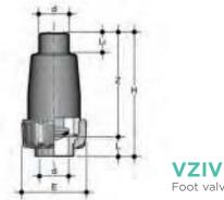
Foot valve with male ends for solvent welding, metric series
