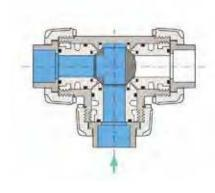
C - T-port ball valve: 180° - Branch closed/direct flow
