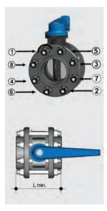
Before tightening the stud-bolts, it is advisable to open the disk in order to prevent damage to the seal. Tighten the stud-bolts in a uniform manner, in the order indicated in the figure, to the operating torque value indicated in the table. The stud-bolts do not need to be excessively tightened in order to produce a perfect hydraulic seal.
