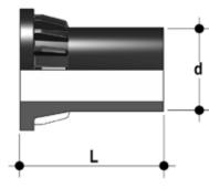
Long spigot PE100 end connectors for joints with electrofusion fittings or for butt welding
