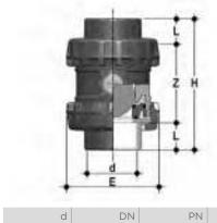
**SXELV** Easyfit ball check valve with female ends for solvent welding, BS series
