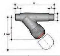
RVDV-RVDT RVDV PVC-U rigid - RVDT PVC-U transparent Sediment strainer with male ends for solvent welding
