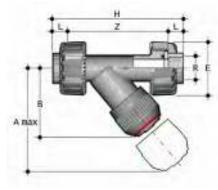
**RVUFV-RVUFT RVUFV** PVC-U rigid - **RVUFT** PVC-U transparent Sediment strainer with BSP threaded female union ends
