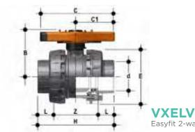
Easyfit 2-way ball valve with female ends, BS series
