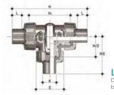
**LKDDV** DUAL BLOCK<sup>®</sup> 3-way ball valve with metric plain spigot ends for solvent welding, L bore
