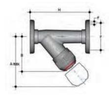
**RVOV-RVOT D 20 ÷ 63 RVOV** PVC-U rigid - **RVOT** PVC-U transparent Sediment strainer with fixed flanges, drilled PN10/16
