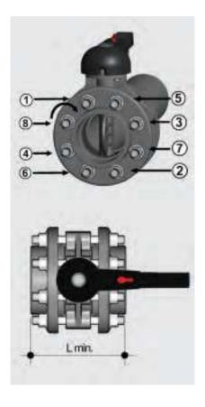
Before tightening the stud-bolts, it is advisable to open the disk in order to prevent damage to the seal. Tighten the stud-bolts in a uniform manner, in the order indicated in the figure, to the nominal operating torque value indicated in the table. The stud-bolts do not need to be excessively tightened in order to produce a perfect hydraulic seal. Overtightening could adversely affect the operating torque of the valve.
