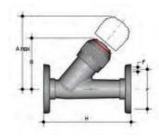
VROV D 20 ÷ 63 Check valve with fixed flanges, drilled PN10/16
