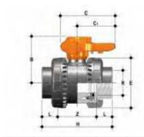
**VXEGV** Easyfit 2-way valve with female ends, JIS thread
