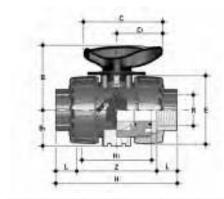
VKRFV DUAL BLOCK<sup>®</sup> regulating ball valve with BSP threaded female ends
