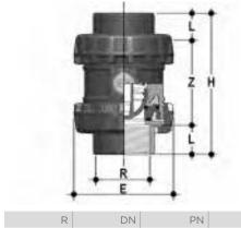
**SSEGV** Easyfit spring check valve with female ends, JIS thread
