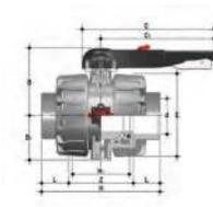
VKDLV DUAL BLOCK® 2-way ball valve with female ends for solvent welding, BS series
