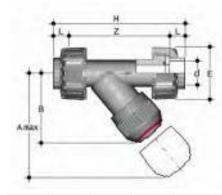
RVUIV-RVUIT RVUIV PVC-U rigid - RVUIT PVC-U transparent Sediment strainer with female union ends for solvent welding
