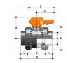
**VXEAV** Easyfit 2-way ball valve with female ends for solvent welding, ASTM series
