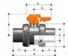
**VXEJV** Easyfit 2-way ball valve with female ends for solvent welding, JIS series
