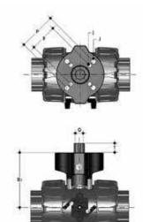
**Power Quick/CE** The valve can be equipped with electric actuators, using the PP-GR module reproducing the drilling pattern foreseen by ISO 5211
