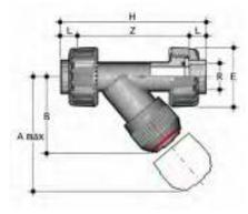
**RVUNT** PVC-U transparent Sediment strainer with NPT threaded female union ends
