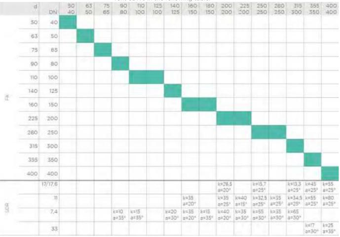
Short/long spigot stubs according to EN ISO 15494 and DIN 16962/16963 and flange
