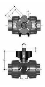
**Power Quick/CE** The valve can be equipped with electric actuators, using the PP-GR module reproducing the drilling pattern foreseen by ISO 5211
