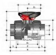
VKDIV/SHX DUAL BLOCK\* 2-way ball valve with handle lock and STAINLESS steel threaded inserts with female ends for solvent welding, metric series
