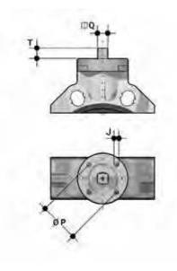
Actuator mounting flange The valve can be equipped with standard pneumatic or electric actuators and gearbox for heavy-duty operations, using a flange in PP-GR reproducing the drilling pattern provided for by standard ISO 5211.
