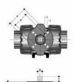
**Power Quick/CP** The valve can be equipped with pneumatic actuators, using the PP-GR module reproducing the drilling pattern foreseen by ISO 5211
