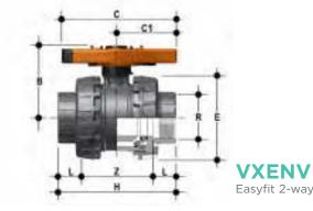
Easyfit 2-way ball valve with female ends, NPT thread
