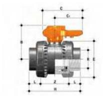
**VXENV** Easyfit 2-way ball valve with female ends, NPT thread
