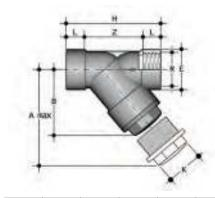
**RVFV-RVFT RVFV** PVC-U rigid - **RVFT** PVC-U transparent Sediment strainer with BSP threaded female ends
