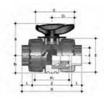
DUAL BLOCK® regulating ball valve with female ends for solvent welding, JIS series
