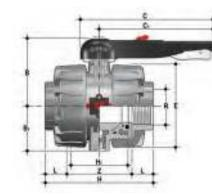
VKDNV DUAL BLOCK<sup>®</sup> 2-way ball valve with female ends, NPT thread
