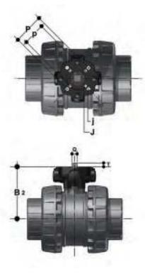
**Power Quick Easyfit** The valve can be equipped with pneumatic or electric standard actuators and gearboxfor heavy-duty operations, using the PP-GR module reproducing the drilling pattern foreseen by ISO 5211.
