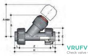
Check valve with BSP threaded female union ends
