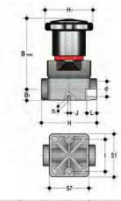
**CMIV** Compact diaphragm valve with female ends for solvent welding, metric series
